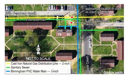
Figure 4. Aerial view showing route of underground utilities near unit 80.
