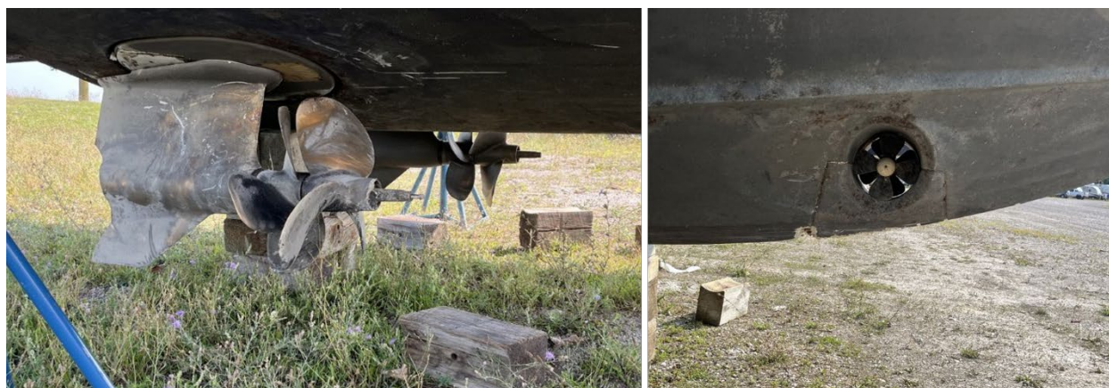
Figure 7. Left to right: Recreational vessel propeller pod damage viewed from the starboard side after the collision, and bow thruster with visible damage to the keel.
