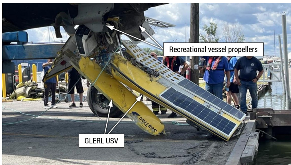
Figure 5. Recreational vessel and GLERL USV hauled out of the water, with the USV split into two large pieces and fouled in the recreational vessel's starboard pod. (Source: Monroe County Sheriff)
