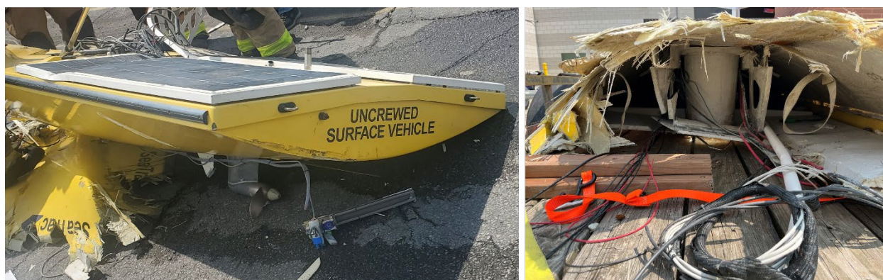
Figure 6. Left to right: GLERL USV after the collision, showing about half of the vessel with its broken fiberglass hull and remaining solar panels intact, and the internal structure of the USV, showing the structural area for scientific equipment and vessel system electrical infrastructure.
