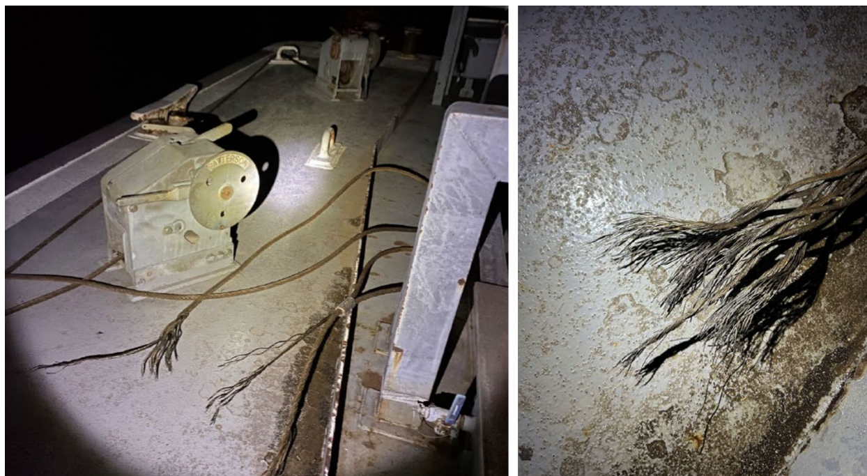
Figure 4. Left to right: Damaged port bow winch wire (headline) located forward on MPC 1056 . (Source: Coast Guard.)
