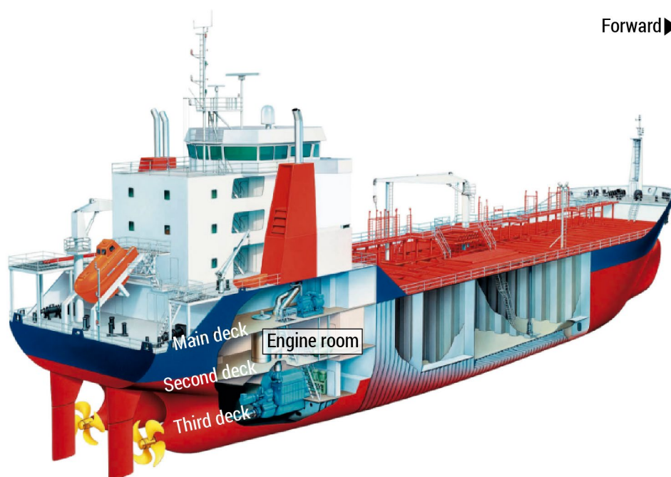
Figure 3. Side profile view of the Scot Stuttgart showing starboard engine room (port engine room similar). (Background source: Scot Stuttgart SA)
