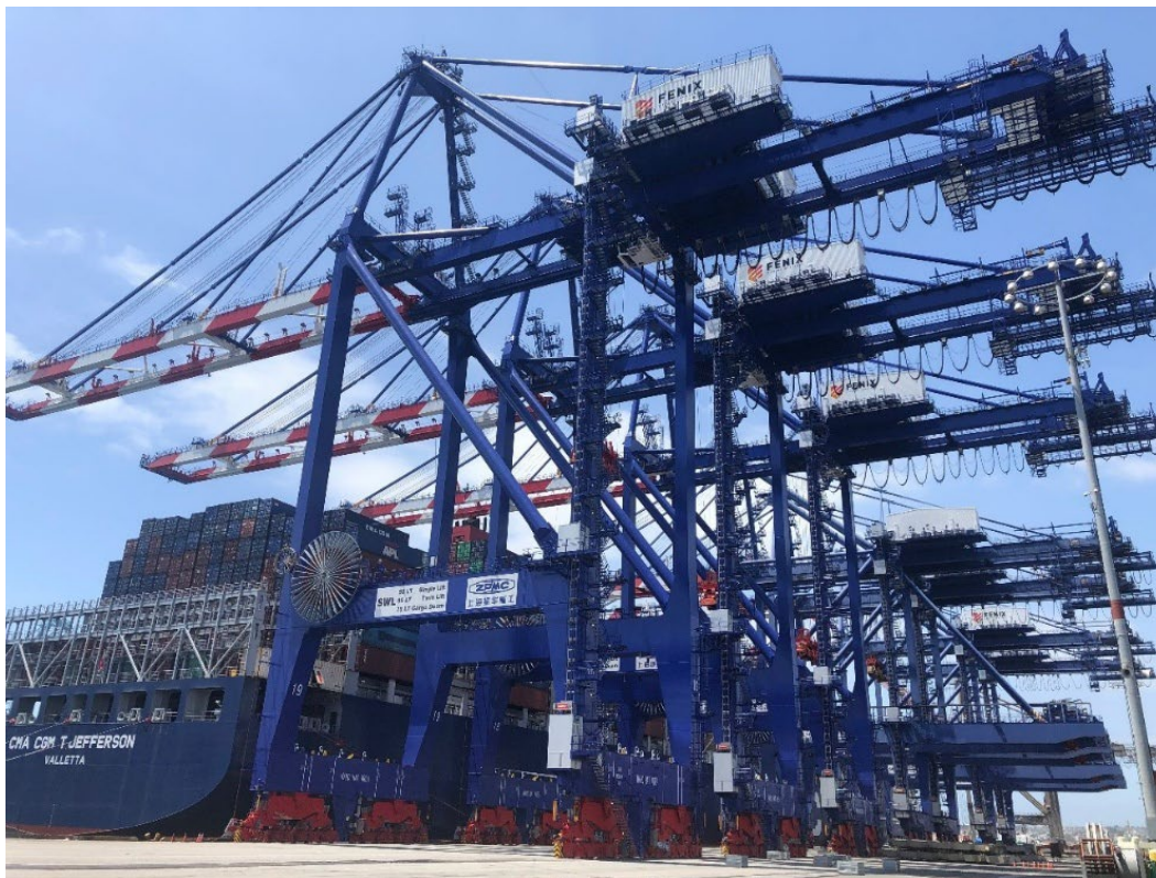
Figure 3. FMS Container Terminal STS cranes with the crane booms in the lowered position. (Source: FMS)
