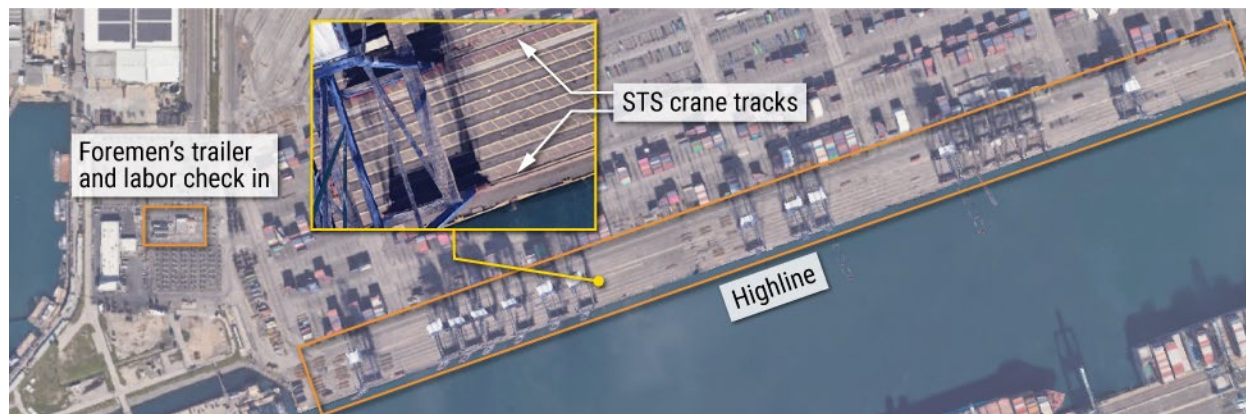
Figure 4. FMS Container Terminal highline and surrounding area. Inset shows the tracks the STS cranes traveled along within the highline. (Background source: Google Earth)
