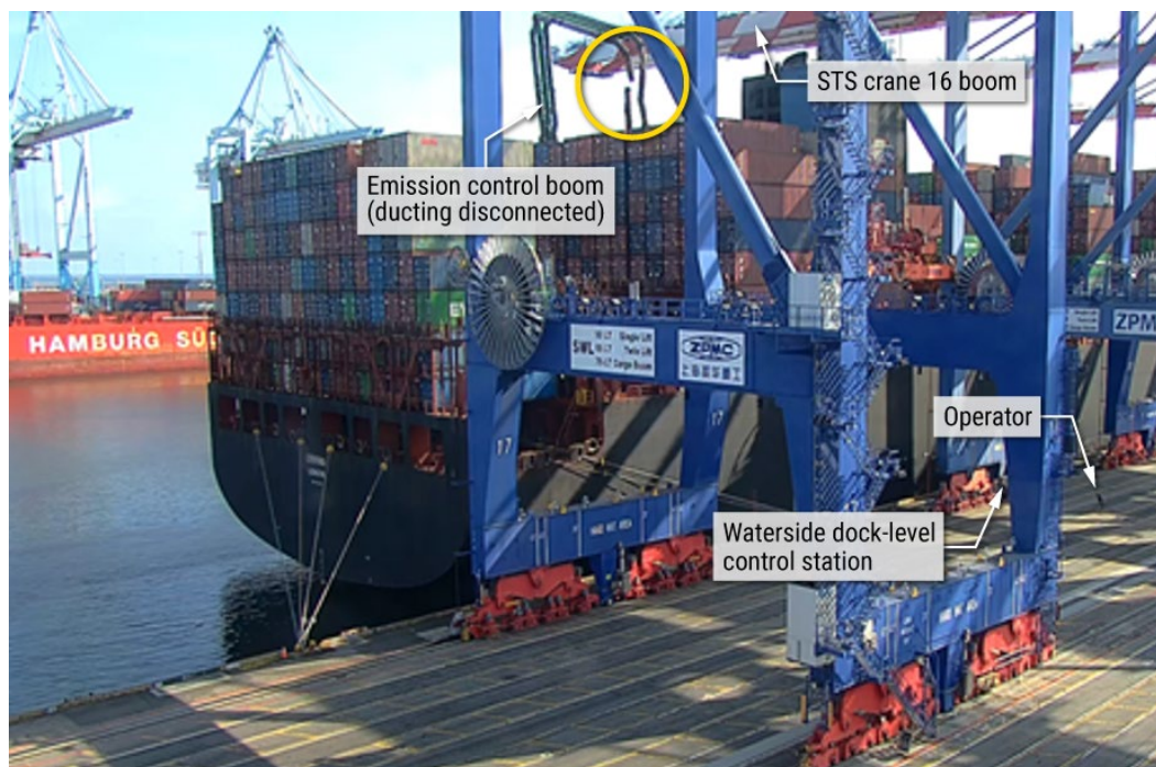
Figure 6. STS crane 16 boom contacting the STAX 1 emissions capture boom (circled) and crane operator 2 running toward the waterside dock-level control station. (Background source: FMS)
