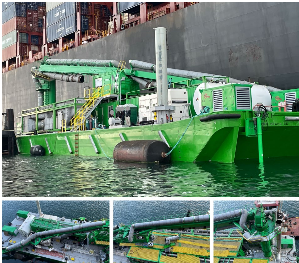
Figure 7. Top: View from the starboard bow of the STAX 1 showing the emission capture boom lying on top of the control room and across the deck. Bottom, from left: Top-down views of the STAX 1 damage from stern to bow, as seen from the starboard side of the Erving . (Source: Coast Guard)
