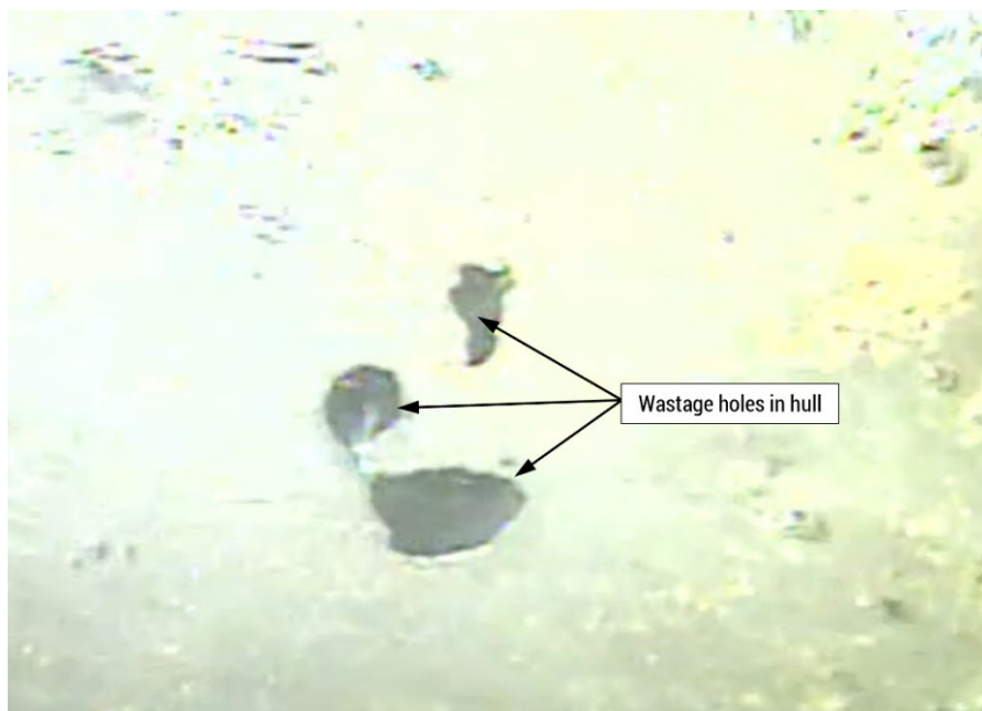
Figure 5. Wastage holes discovered in hull during postcasualty survey. (Background source: Global Diving)
