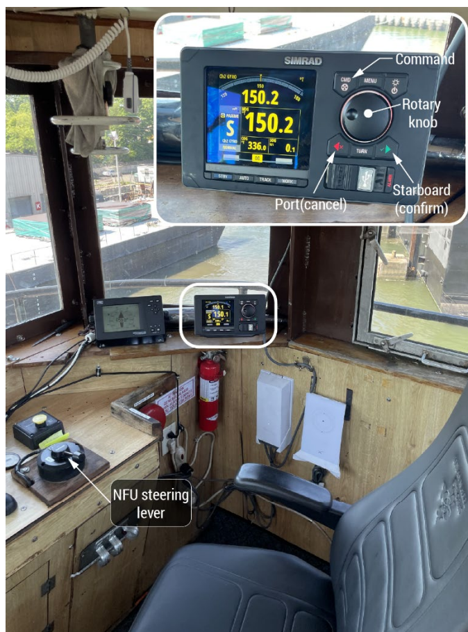
Figure 9. Starboard side of Mackenzie Rose upper wheelhouse with autopilot controller after the casualty.
