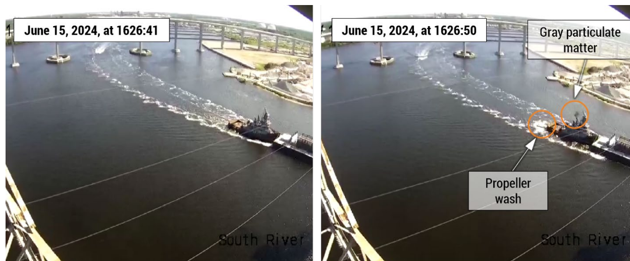
Figure 11. From left to right: CCTV footage of Mackenzie Rose tow at time of contact, and 9 seconds after the contact, showing propeller wash and gray exhaust particulate matter from vessel's exhaust stack. (Background source: Norfolk and Portsmouth Belt Line Railroad Bridge)
