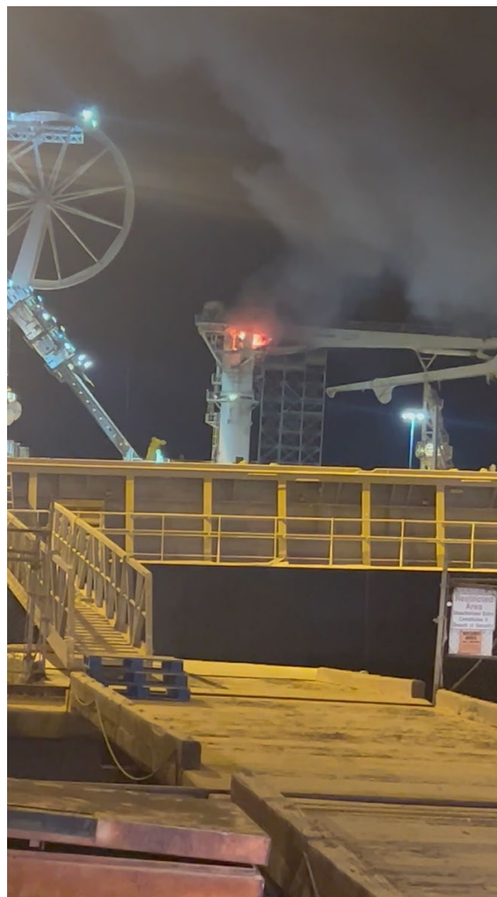
Figure 4. The crane cabin on fire, as seen from shore, after the fire broke the glass and before the arrival of the Mobile Fire Department. (Source: Unknown, via Coast Guard)
