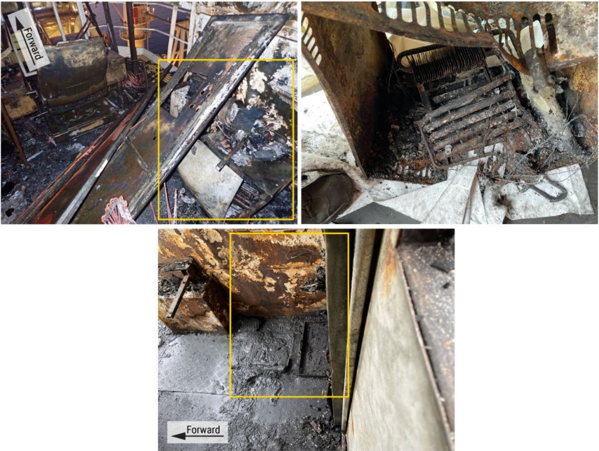
Figure 6. Top: The crane cabin interior after the fire, with the location of the refrigerator and other objects outlined in yellow, and the burnt remains of the refrigerator. Below: The fire pattern on the bulkhead and damage to the deck underneath the removed refrigerator outlined in yellow. (Background source [ top left ]: Coast Guard)
