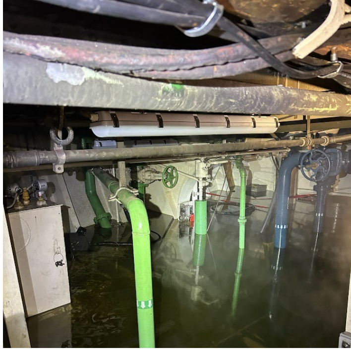
Figure 5. The engine room within the Cuyahoga following the water ingress. (Source: Coast Guard)
