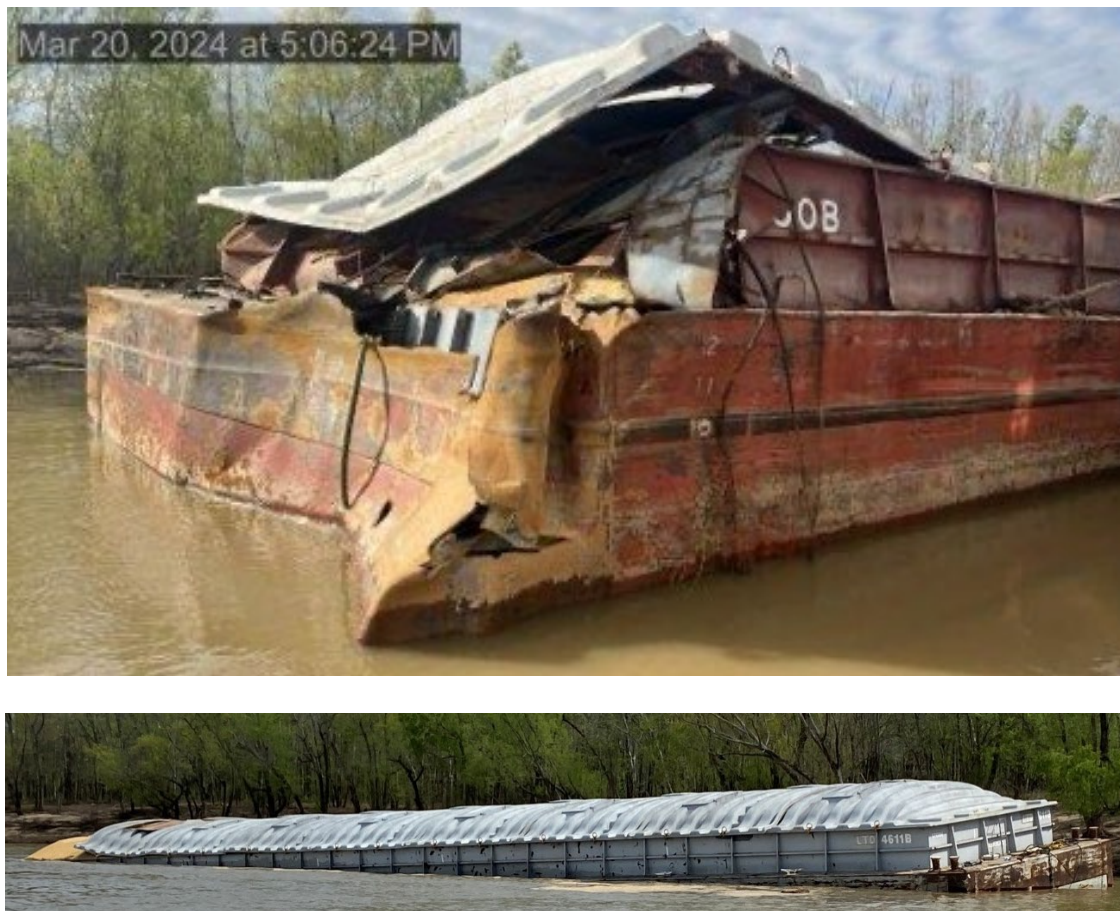
Figure 6. From top: Damage to the stern area of MTC 500B , the barge that was immediately aft of the PTC 706 , and covered barge LTD 4611B partially sunken by its bow to port. (Source: Budwine and Associates, LLC)
