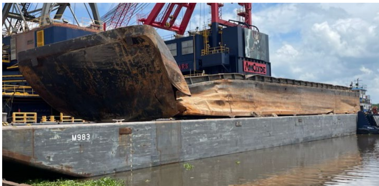
Figure 7. Barge PTC 706 after arriving at the recycling yard in Houma, Louisiana, on April 22, 2024, with damaged rake. (Source: Modern American Recycling Services, Inc.)
