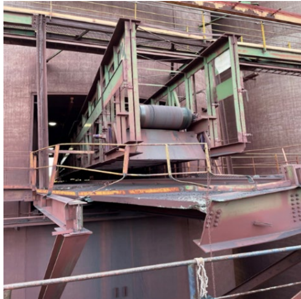
Figure 4. Damage to one of the loading shuttles at the BNSF Allouez Taconite Facility following the casualty. (Source: Coast Guard)
