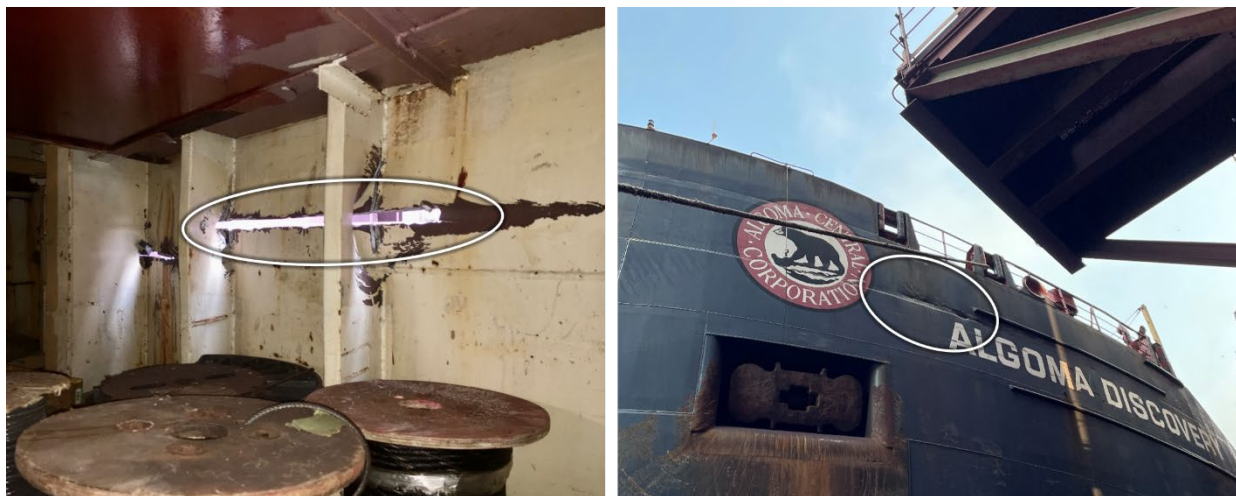
Figure 5. Left to right: Damage (circled) to the Algoma Discovery , as seen from the interior and the exterior, following the casualty. (Source: Coast Guard)
