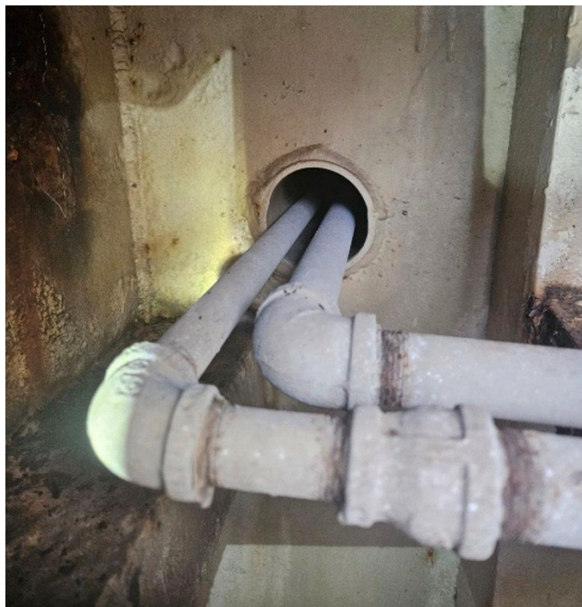
Figure 6. View of unsealed conduit penetration between the engine room and auxiliary space from the auxiliary space on May 28, 2024. (Source: Coast Guard)
