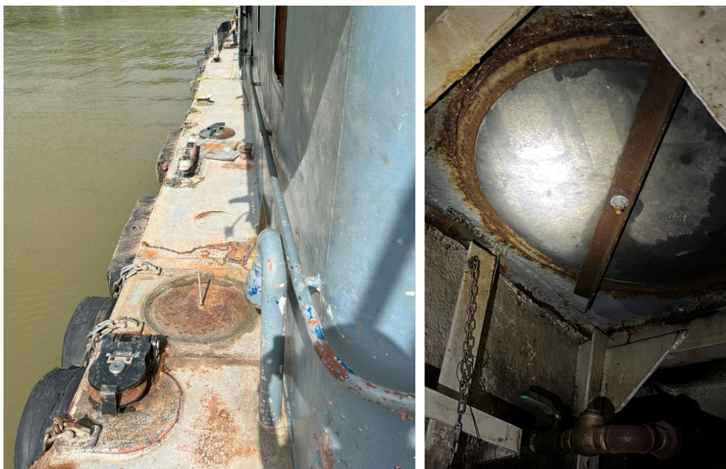
Figure 5. Cajole after the sinking, with starboard side auxiliary void access hatch cover replaced and permanently sealed to the main deck for transit to shipyard.
