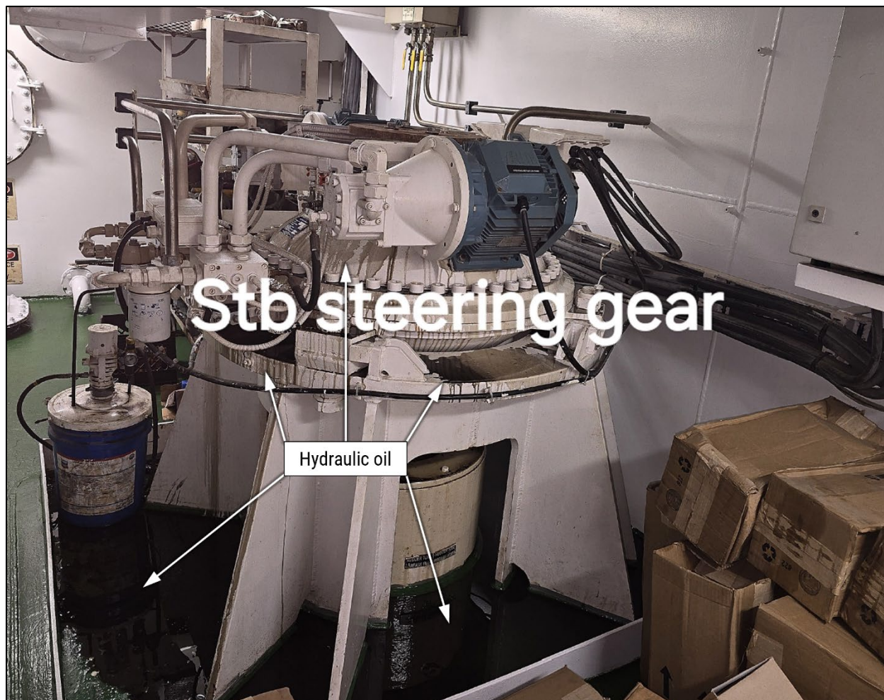
Figure 7. Jack Edwards starboard steering gear as found immediately after collision. (Background source: ECO)
