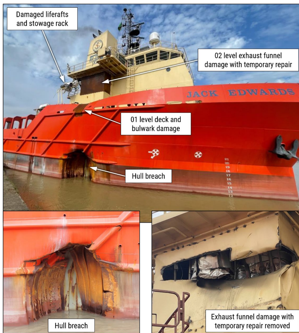
Figure 8. Jack Edwards external damage. (Source: ECO)
