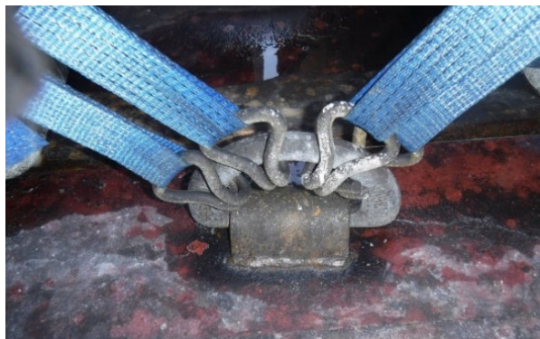
Figure 7. Postcasualty photo showing a D-ring held by a bracket that is attached to the tween deck, with four hooks (two lashing belts). (Source: Coast Guard)
