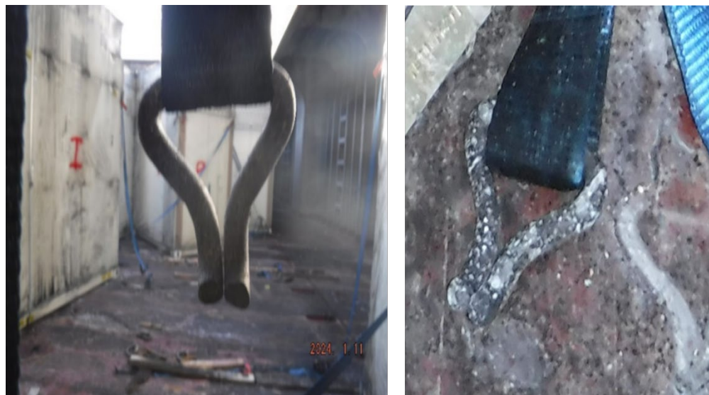
Figure 15. Photos of two separate hooks that fractured and separated from a D-ring. (Source: Coast Guard)
