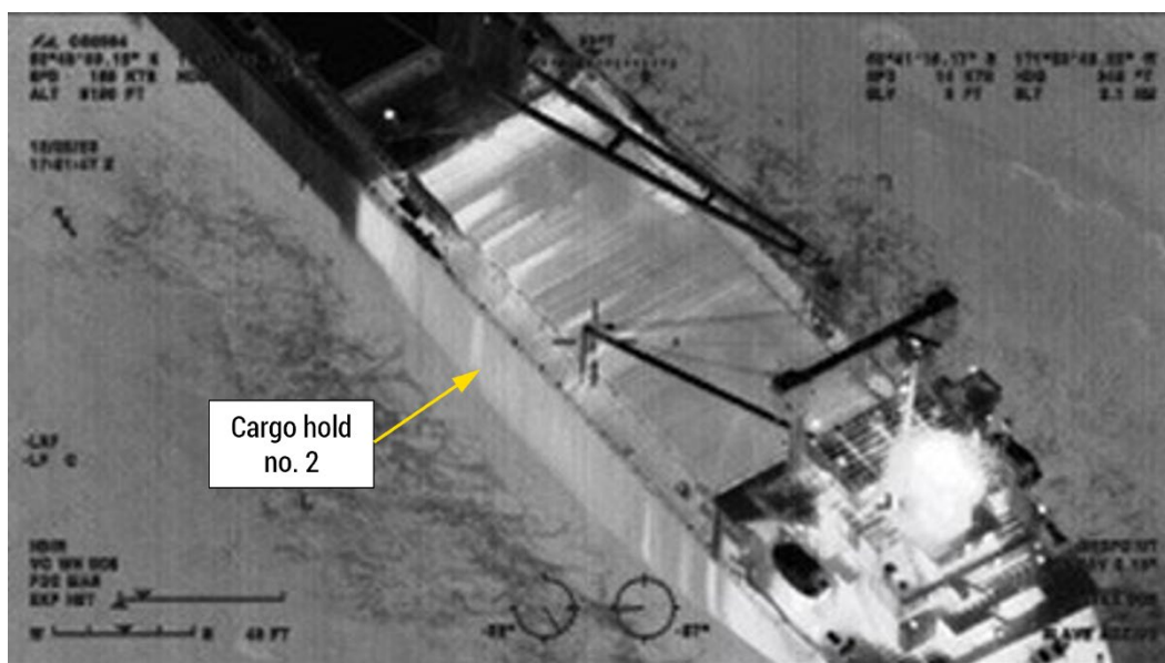
Figure 8. Infrared photo of the Genius Star XI en route to Dutch Harbor, showing an indication of heat (in white) within cargo hold no. 2 on December 28. (Background source: Coast Guard)
