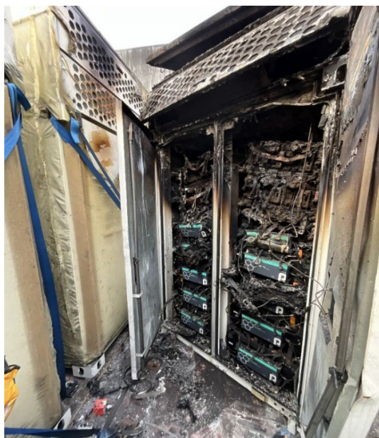
Figure 16. Example of a BESS unit with internal fire damage. (Source: ESA)
