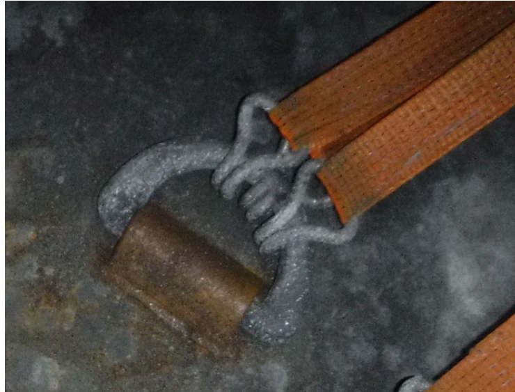
Figure 14. Example of hooks and lashing belts holding a HARPS Heat Exchanger, with only the tip of the hook in contact with the D-ring. (Source: Coast Guard)
