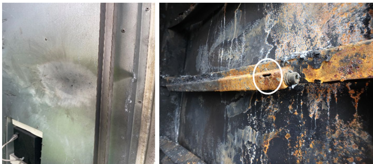
Figure 22. Left to right: Examples of internal damage due to indent and scorching, and arcing (circled) found inside of the BESS units on the tween deck in cargo hold no. 1 and no. 2. (Background source: ESA)
