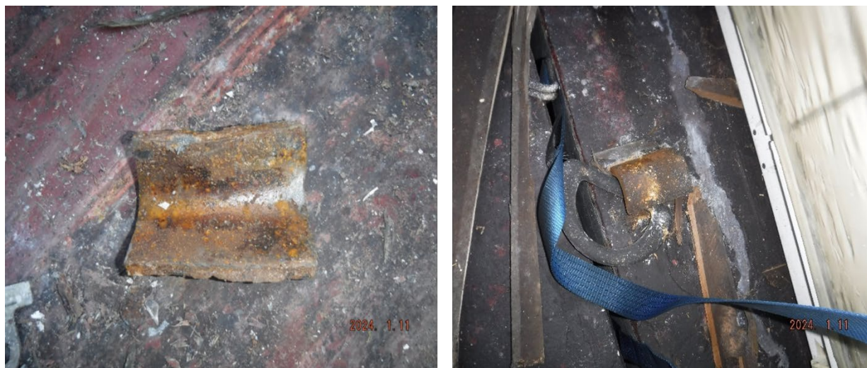
Figure 12. Left to right: Bracket found separated from the deck, and a D-ring partially pulled from a deformed bracket that was still connected to the deck. (Source: Coast Guard)
