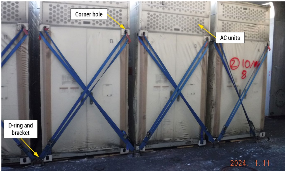
Figure 6. Postcasualty photo showing the method used to secure the units within the cargo hold. (Source: US Coast Guard).
