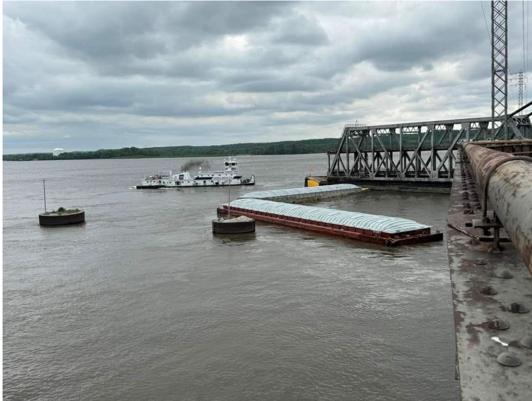
Figure 6. Barges IN122011 and IN155499 immediately after impact blocking the primary channel. The IN155499 , next to the central wooden fendering, sinking. The Joe B. Wyatt is visible in the background. (Source: Coast Guard)
