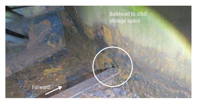
**Figure 8.** Rust, rust scaling, water accumulation markings, and a wastage hole (circled in white) in the transverse bulkhead between the starboard aft void (inboard forward corner) and the starboard storage room forward of it (viewed from the starboard aft void)
