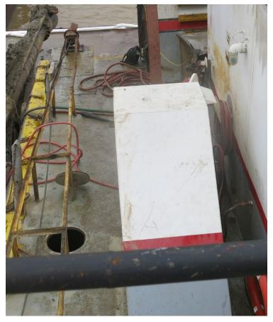
**Figure 7.** Postrecovery photo showing the flush hatch for the starboard aft void. Hatches were opened for salvage operations.
