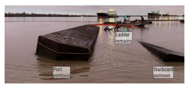
**Figure 5.** The overturned hull of the WB Wood with its port pontoon on the left and the starboard pontoon on the right the morning after the capsizing. (Source: US Coast Guard)
