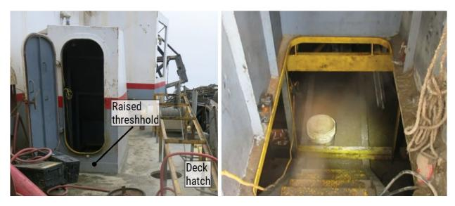
**Figure 4.** Postrecovery photos of the door to the starboard storage space and the starboard aft void deck hatch, viewed from the starboard aft main deck looking forward (*left*), and the storage space interior from the main deck door looking down and forward (*right*).
