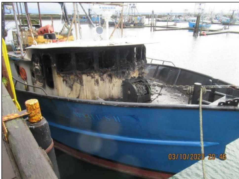
Figure 3. The burned-out Marlins II after the fire. (Source: Blomquist Marine Surveys)
