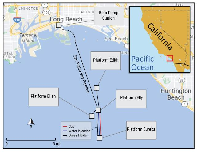
Figure 2. Simplified illustration of the San Pedro Bay Pipeline and supporting structures.
