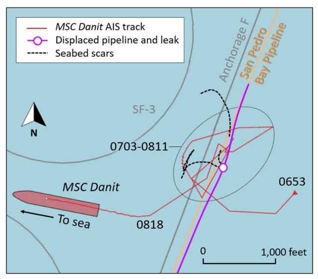
**Figure 25.** The *MSC Danit*'s AIS data indicated that the vessel maneuvered directly over the pipeline and remained there for over an hour.
