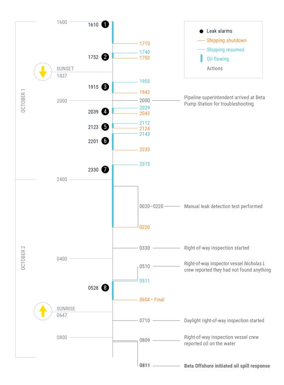
Figure 3. Timeline of leak alarms and oil release discovery.
