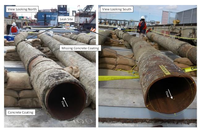
**Figure 17.** Opposite ends of the pipe segment that contained the leak site, which had been temporarily repaired with a welded repair patch, visible in the right image. Damage signatures observed included lateral deformation, out-of-roundness deformation (a typical example indicated at the end of the segment in the right image), and missing concrete coating, especially north of the leak site.
