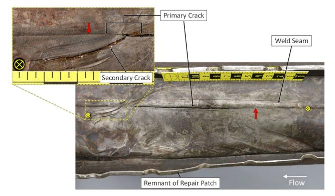
**Figure 18.** A closer view of the leak site from the outer surface after removal of the repair patch showing general inward deformation, localized gouges, parallel scratches, and smeared metal. The red arrows mark the ends of a visible primary crack along the seam weld toe. The two holes denoted by a yellow circled *X* were introduced following underwater nondestructive testing to prevent further cracking. Inset scale markings are 0.25 inches.
