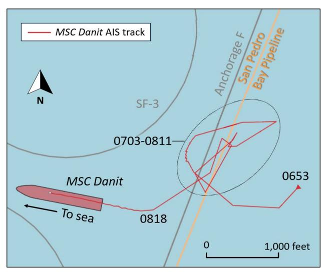
Figure 14. AIS track of the MSC Danit between 0653 and 0818.
