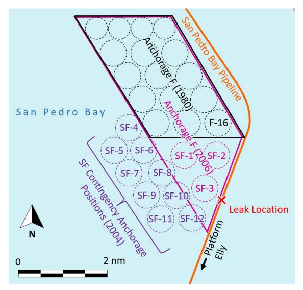
**Figure 15.** Boundaries of Anchorage F, as originally drawn in 1980 (in black) and as revised in 2006 (in magenta). Also shown are nine contingency anchorage positions established in 2004 (in purple). (Other contingency anchorages in San Pedro Bay are not shown.) (Background source: Google Maps)
