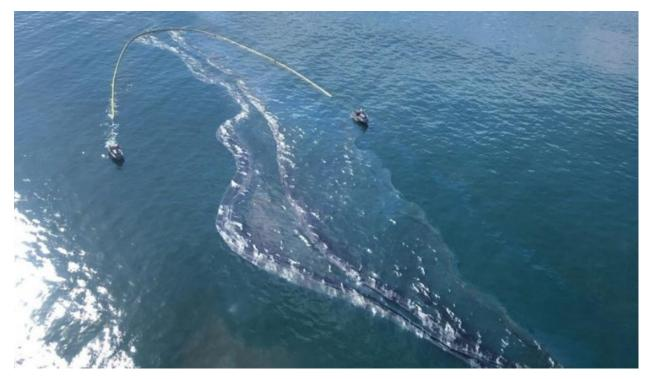
**Figure 1.** Crude oil in the Pacific Ocean off the California coast on October 3, 2021. Oil spill removal organization vessels are towing a skirted oil boom to contain the oil spill. (Source: US Coast Guard)
