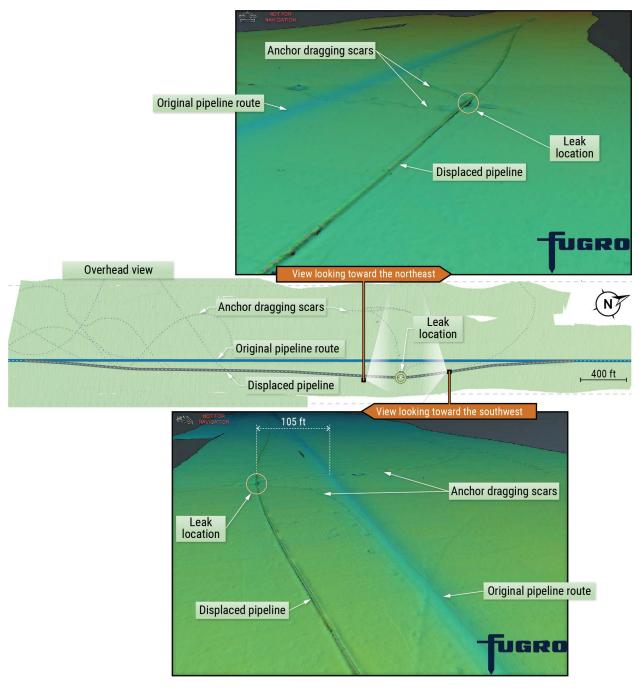
**Figure 5.** Results of the survey showing the San Pedro Bay Pipeline original location, leak location, pipeline displacement, and anchor dragging scars, viewed looking toward the northeast (*top*), from overhead (*middle*), and looking toward the southwest (*bottom*). (Background sources: Amplify, Aqueos, Fugro)
