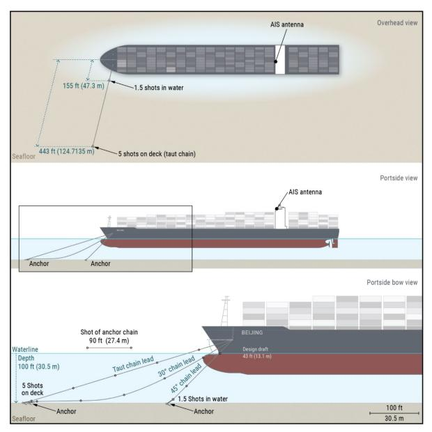
**Figure 20.** NTSB modeling of *Beijing* anchor position relative to the vessel for moderate to heavy strain on the anchor chain. (In the profile views, the anchor chain is shown tending directly ahead of the vessel for illustrative purposes.)
