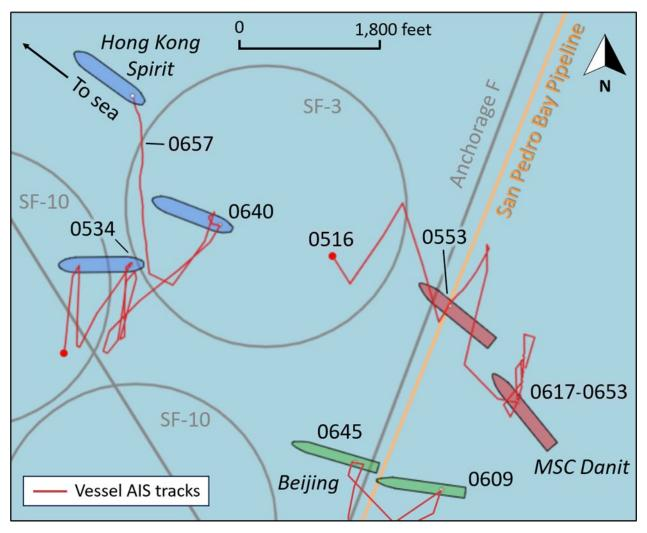
**Figure 13.** Initial AIS track of the *MSC Danit* as it moved out of anchorage position SF-3 and crossed the charted location of the San Pedro Bay Pipeline. Also shown is the AIS track of the *Hong Kong Spirit* as it dragged anchor into the *MSC Danit*'s assigned anchorage, and the AIS track of the *Beijing* as it dragged anchor off the port side of the *MSC Danit*, during the same period. (See figure 14 for remaining track of *MSC Danit* during anchor dragging.)
