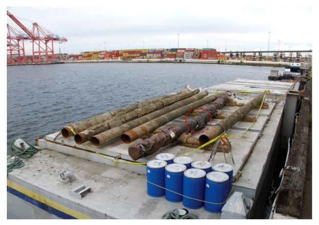
**Figure 16.** Six segments of damaged pipeline removed for replacement. The leak site, circled in red, was observed on the segment shown wrapped in a tarp.
