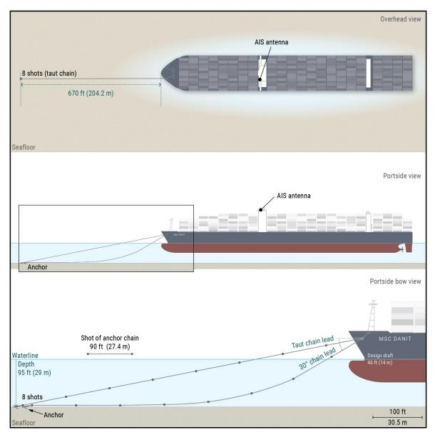
**Figure 23.** NTSB modeling of the *MSC Danit*'s anchor position relative to the vessel for moderate to heavy strain on the anchor chain.
