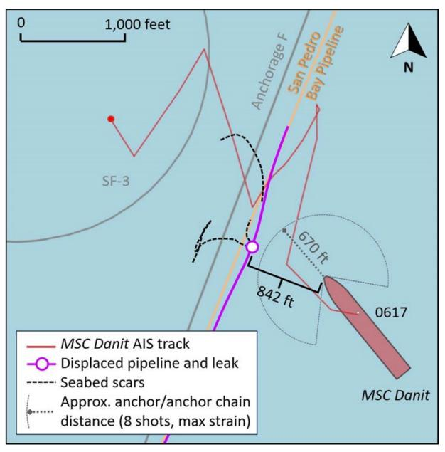
**Figure 24.** The *MSC Danit*'s position as the vessel dragged anchor over the San Pedro Bay Pipeline, the approximate distance of the anchor from the vessel, and location data from anchor dragging scars on the seabed.
