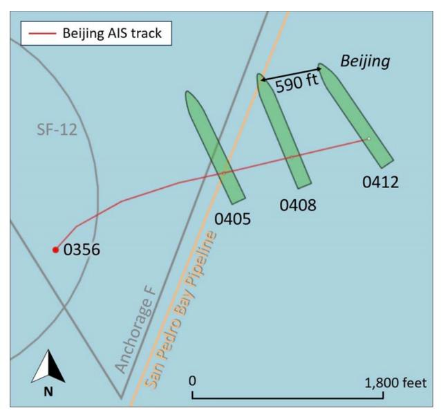
**Figure 11.** Initial AIS track of the *Beijing* as it moved out of anchorage position SF-12 and crossed the San Pedro Bay Pipeline on January 25, 2021. (See figure 12 for full track of the *Beijing* during anchor dragging.)
