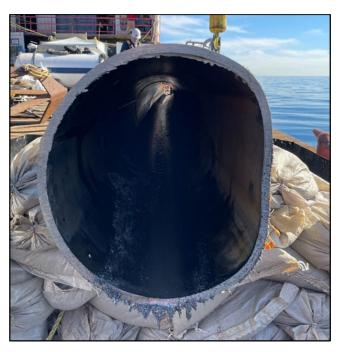
**Figure 19.** End of segment that had been located along the displaced length of pipeline to the south of the leak locations, showing out-of-roundness deformation. (Source: PHMSA)
