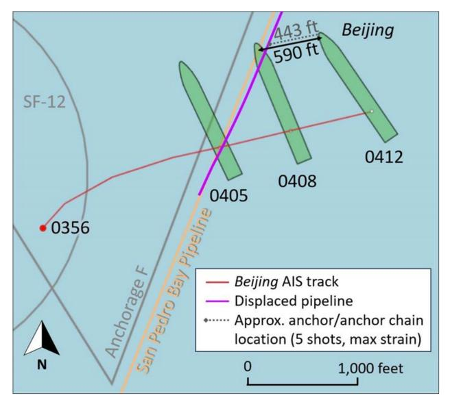
**Figure 21.** The *Beijing*'s position as the vessel dragged anchor over the San Pedro Bay Pipeline.
