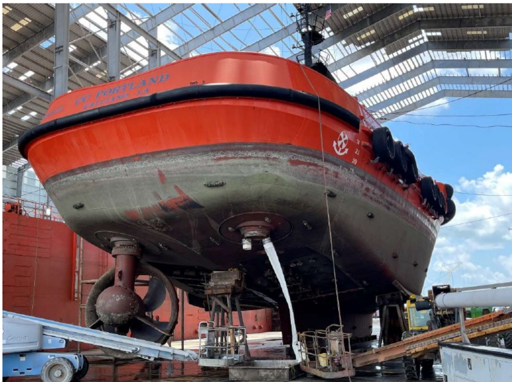
Figure 6. The CC Portland in drydock showing the missing starboard Z-drive unit. (Source: Coast Guard)
