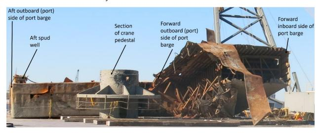
**Figure 7.** The two sections of barge *GD 962* (the *Ambition*'s port barge) after recovery from the Gulf of Mexico.
