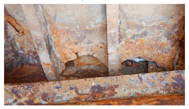
**Figure 7.** The bottom of the centerline longitudinal bulkhead between the no. 1S and no. 1P compartments of the port barge showing metal loss and corrosion holes. (Source: K. Smith Marine Surveying)
