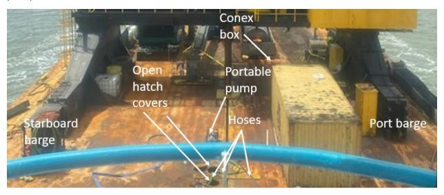
**Figure 5.** The barge *Ambition* at 1200 on June 14 while being pushed southbound on the Calcasieu River en route to the fuel facility. A portable pump and hoses are visible leading into open hatches on the deck of the starboard barge near the bow on the inboard side, with a discharge hose leading out onto the main deck. (Source: *Karen Koby* mate)
