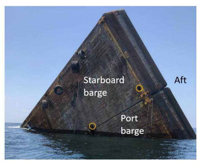
**Figure 6.** The partially sunken barge *Ambition* the morning of the casualty with the starboard stern of the barge out of the water. The orange circles show hatch covers that had fallen off during the capsizing. (Background source: unknown)
