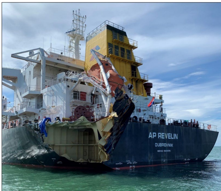
Figure 5. Damaged stern area of the AP Revelin after the collision.
