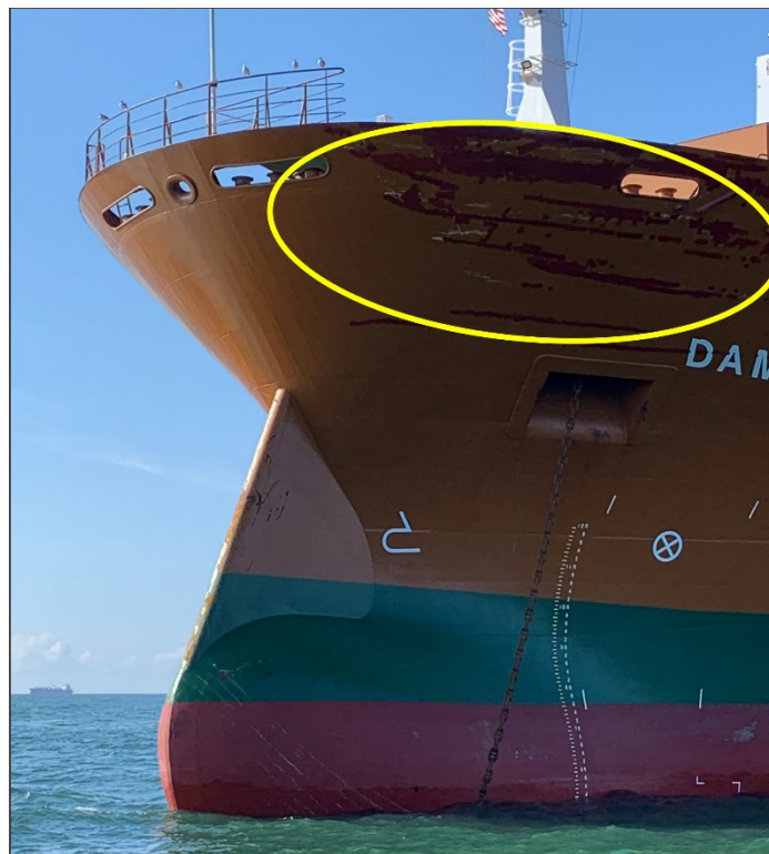
Figure 6. Port bow of the Damgracht after the collision with damage circled in yellow.
