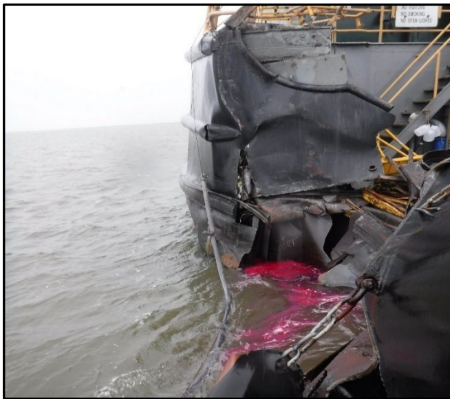
The port side of the Cheramie Bo Truc No 22 , post-collision, showing the compromised no. 1 port fuel tank and oil spillage. (Source: Coast Guard)
