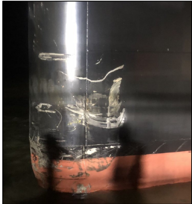
Damaged stem of the barge Texas . (Source: Moran Towing Corp.)
