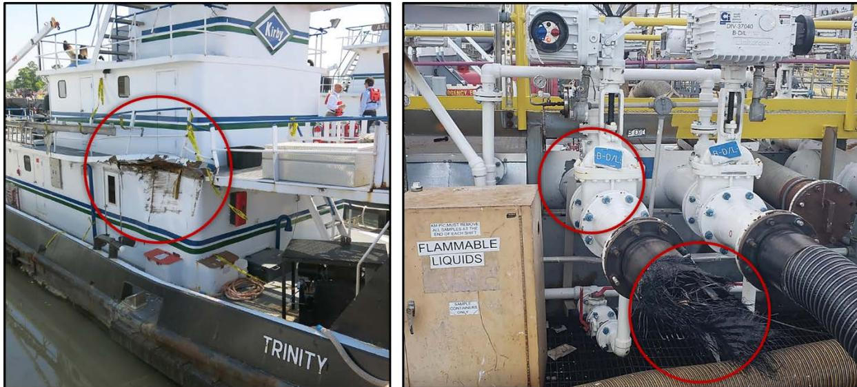
**Left:** Damage to the *Trinity*'s starboard side from the impact of barge *Kirby 29751*. **Right:** Damaged shoreside cargo hose and deformed piping at the manifold at the Kinder Morgan facility. (Source: Kinder Morgan Pasadena Liquids Terminal)
