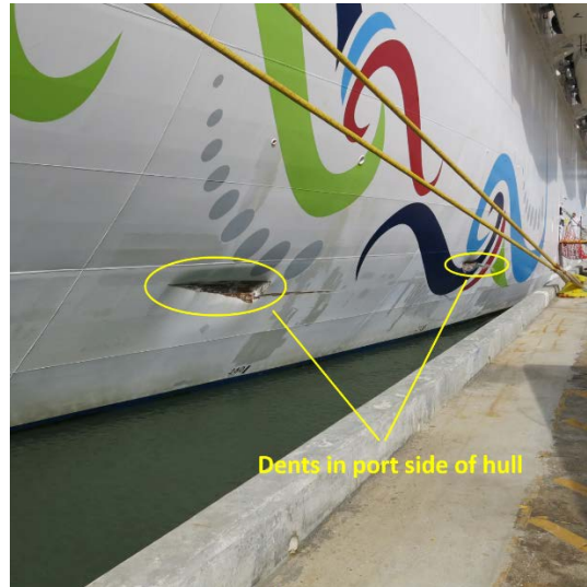
Damage to the Norwegian Epic 's hull.
