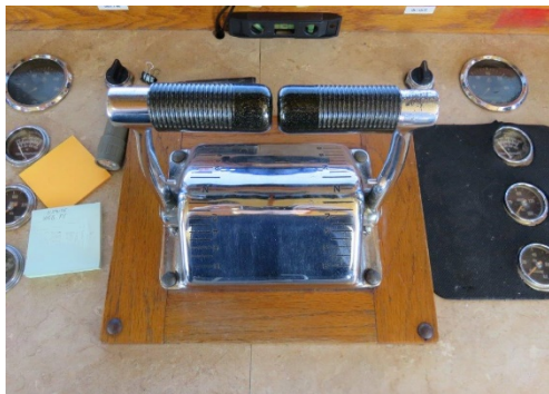
Wheelhouse console engine throttle levers used to control each engine's speed and transmission.
