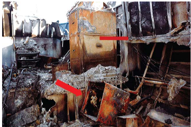
Forward starboard corner of the upper passenger compartment: the red horizontal line represents the location of the chest freezer before the fire, and the red arrow points to the remains of the chest freezer on the deck of the crew quarters. (Source: SEA, Ltd.)
