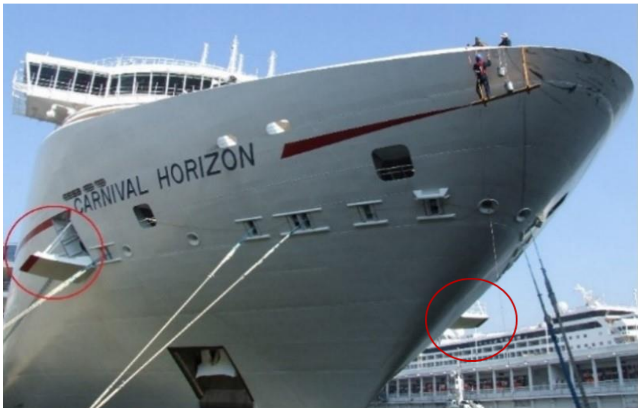
Carnival Horizon's bow after the accident. The forward mooring platforms where the lookout was stationed (about a 100 feet aft from the tip of the bow) are circled in red. (Source: Coast Guard)
