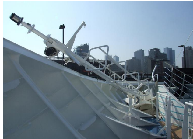
Left, screenshot from Carnival Horizon 's thermal night-vision bow camera at the time of impact with Pier 90. Right, Carnival Horizon 's damaged forward mast and support structure.
