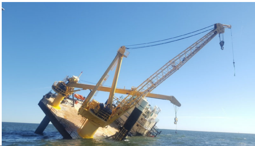
The Ram XVIII after the vessel was abandoned, showing a significant angle of inclination to port. (Source: Coast Guard)
