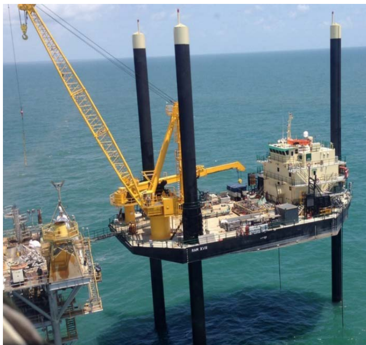
The liftboat Ram XVIII elevated at a previous work site. (Source: Aries Marine)
