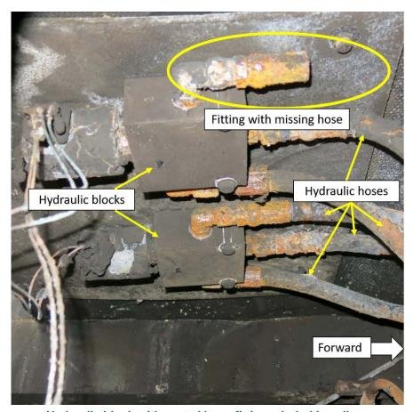
Hydraulic block with parted hose fitting, circled in yellow.
