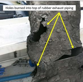
Left: Damage to the engine as seen from above. Right: Damaged exhaust tubing after removal from engine room.
