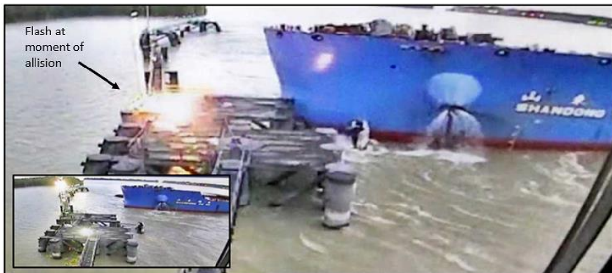
Initial impact of the Shandong Fu En bow swinging into the Ergon-St. James Terminal wharf at 0637:08. Inset: Screenshot of the Shandong Fu En 20 seconds earlier. A crack and three other holes were found in the bulk carrier's shell plate below the waterline. (Video by Ergon-St. James Terminal)
