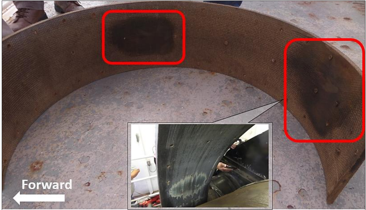
Photo of the upper brake band liner for the starboard anchor. Highlighted in red are the friction marks on the liner. The inset shows the paint worn from heat accumulation through the liner aft section of the upper band.
