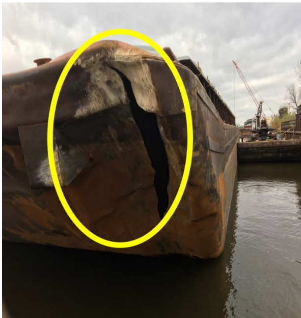
Damage from allision: (at left) raked bow of port lead barge, ART 35157 ; (at right) fixed pier of swing bridge near left descending bank struck by barge (downstream view).
