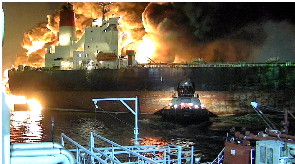
Aframax River after the allision with dolphin no. 78B. Tractor tugboat David B is in the foreground rendering assistance. (Image courtesy of ITC City Dock security video)
