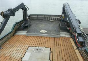
At left is the aft main deck of the *Ambition*, viewed from the stern, showing rectangular bolted hatches for the forward and aft fish holds with access hatches inset. At right is the aft deck, viewed from the deckhouse, showing access hatches to the lazarette and potable-water tank.
