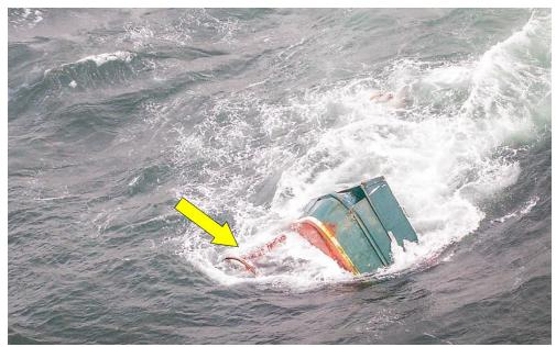
Starboard aft quarter of the *Ambition* prior to final sinking. Arrow shows part of net guard installed to protect the propeller and rudder. (Photo by Coast Guard)
