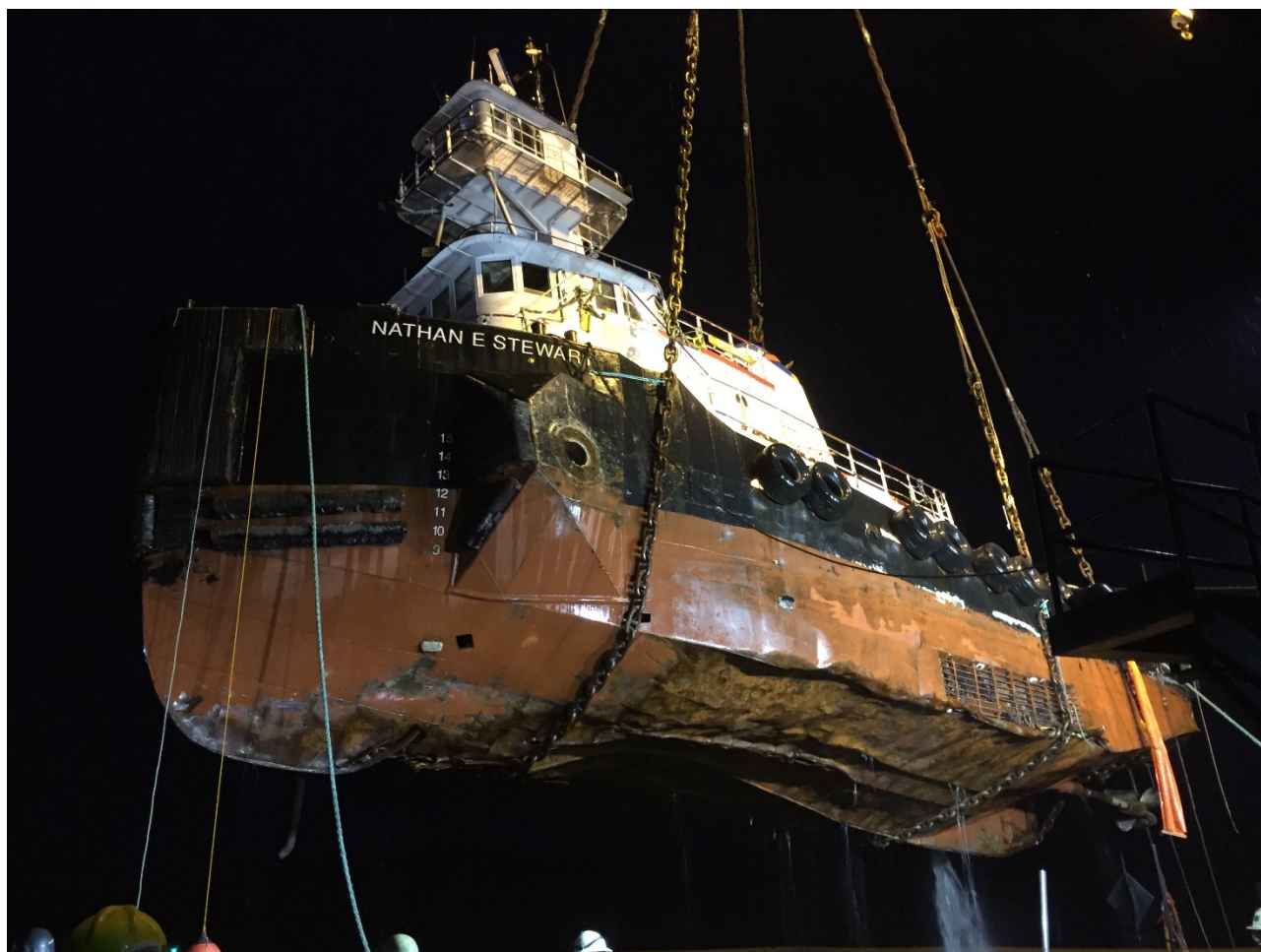
Nathan E Stewart , shortly after being hoisted by the heavy-lift floating crane D.B. General . (Photo by Kirby Offshore Marine)
