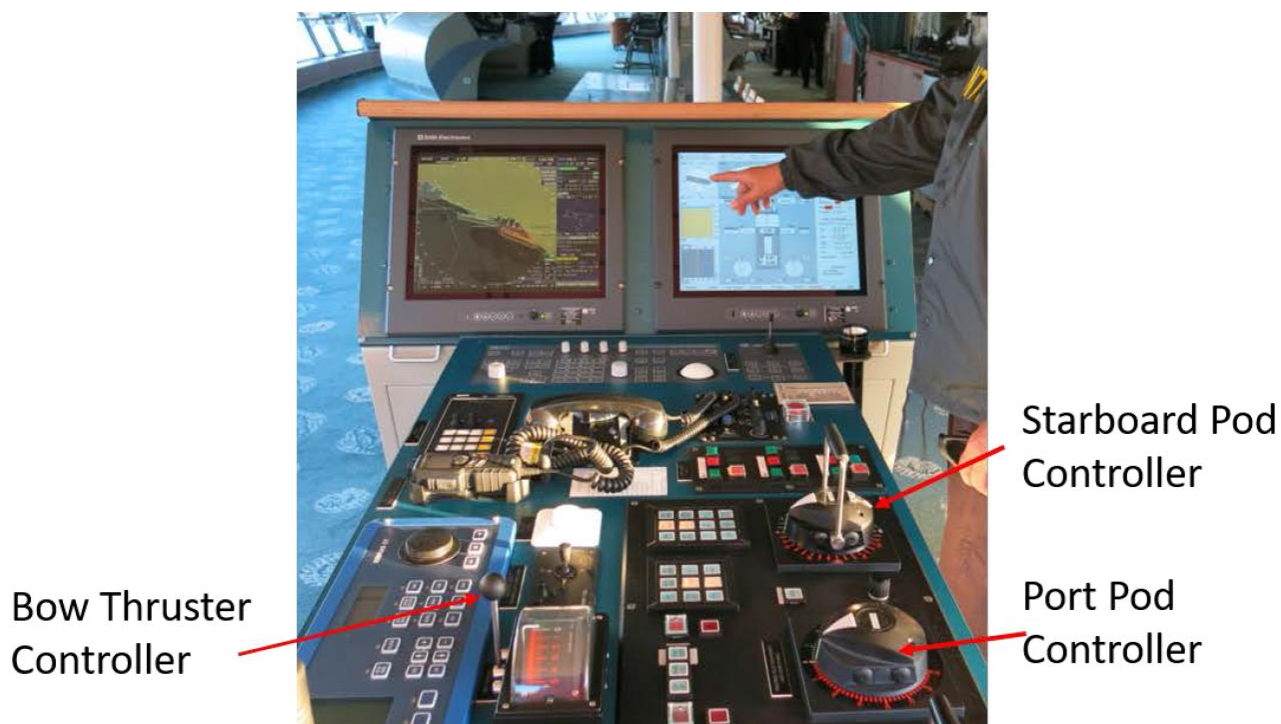
Celebrity Infinity's port bridge wing conning console (the handle to the port pod controller is missing in this photo).
