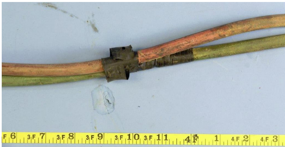
Recovered hose with evidence of repairs consistent with electrical tape. The entire lengths of both hose sections showed signs of degradation.
