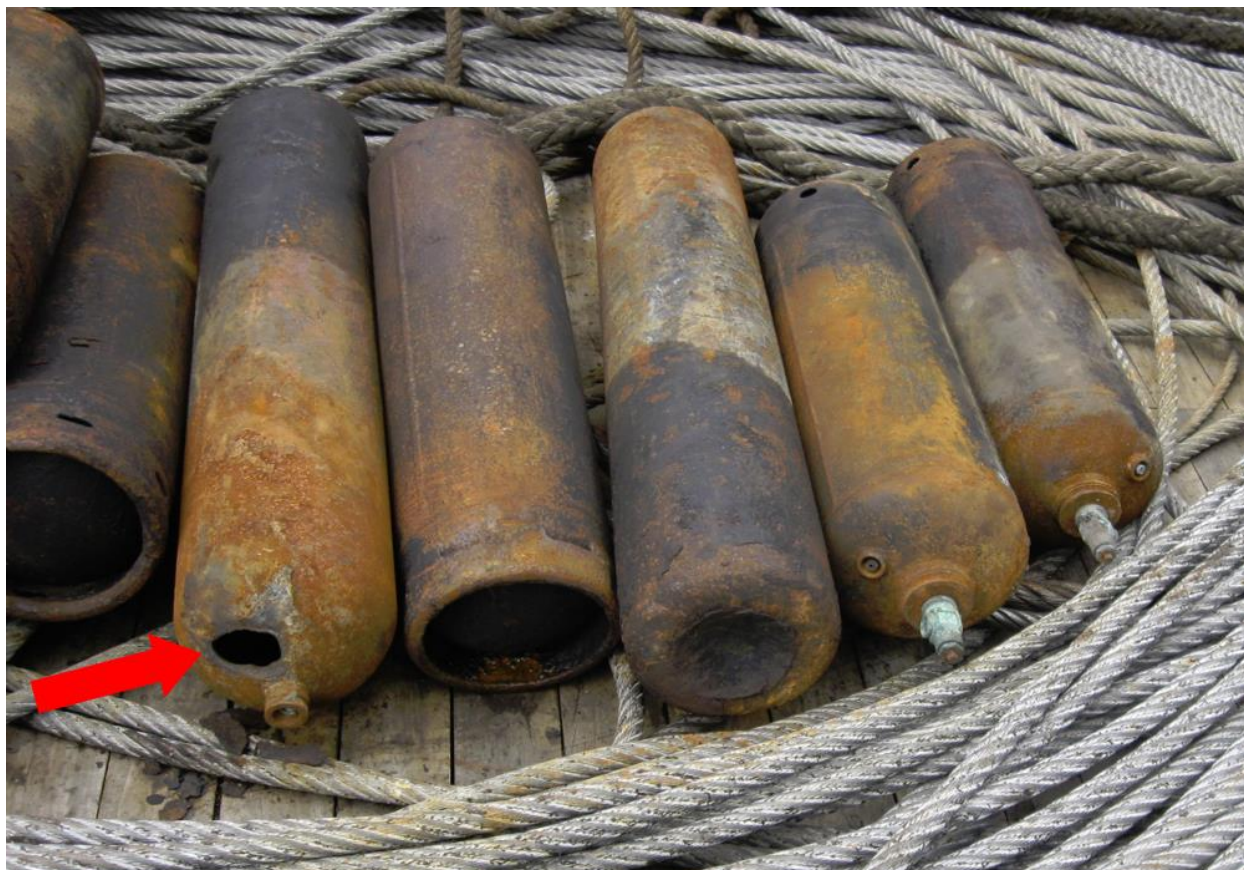
Oxygen and acetylene bottles on deck post-fire. Arrow shows a hole at the melted pressure-relief fusible plug location on one of the bottles. (Photo by Coast Guard)
