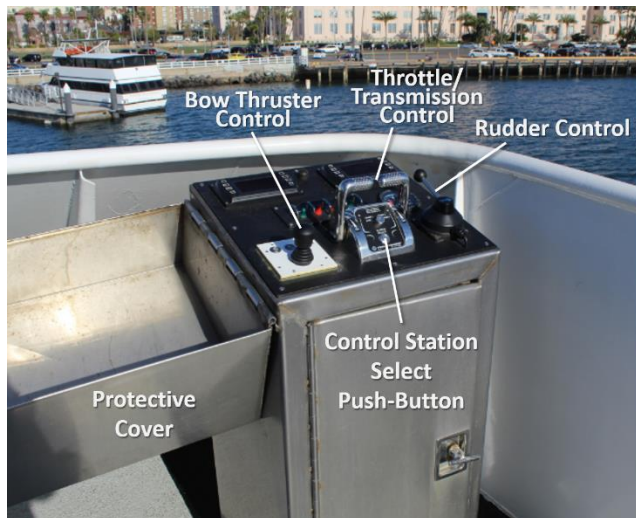
Starboard wing station control box.
