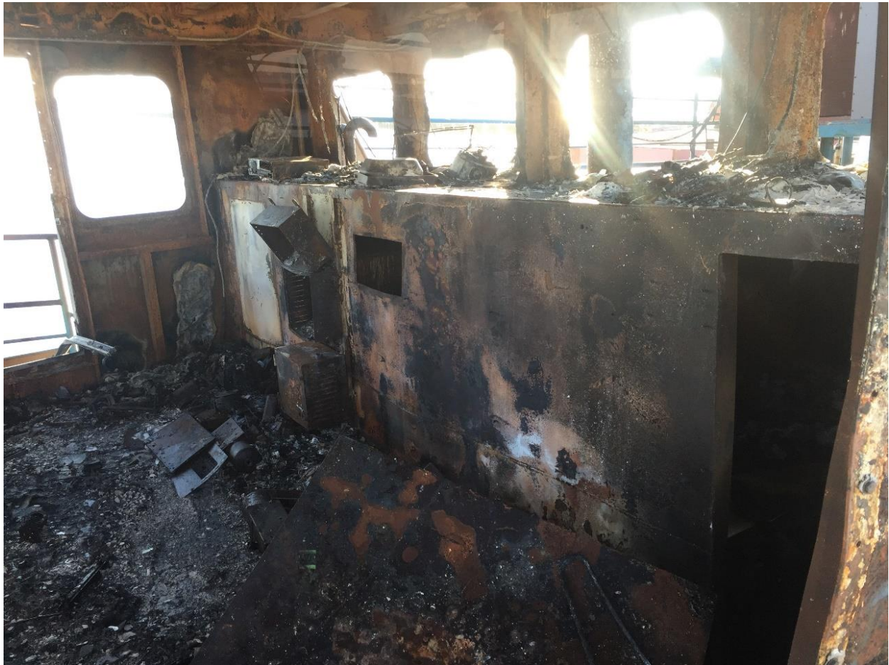
Thomas Dann's wheelhouse after the fire, showing the aft starboard bulkhead. (Photo by Coast Guard)
