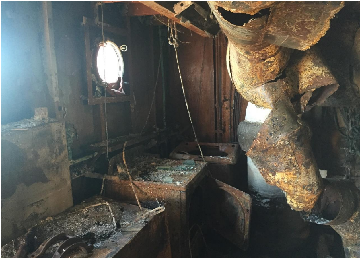
The upper engine room where the fire was determined to have originated. (Photo by Coast Guard)
