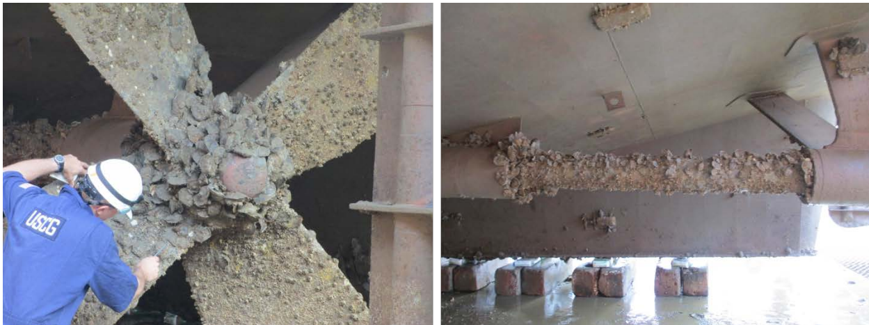
At left, a Coast Guard inspector examines the condition of the port propeller. At right, marine growth on the port tail shaft. (Photos by Coast Guard)
