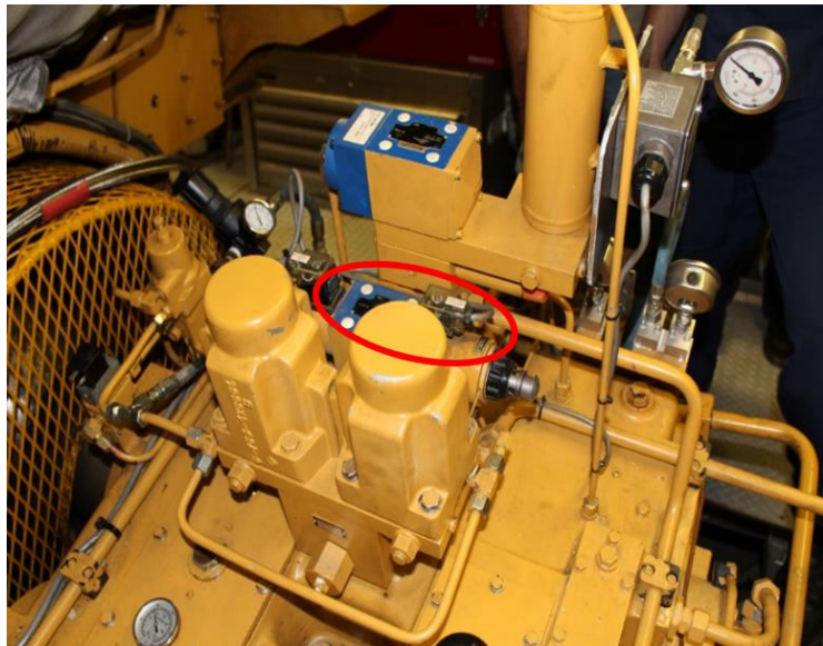
Reintjes starboard engine reduction gearbox. The astern wiring harness on the electronic selector valve solenoid had loose 12-volt wires at the terminal connection, circled in red.
