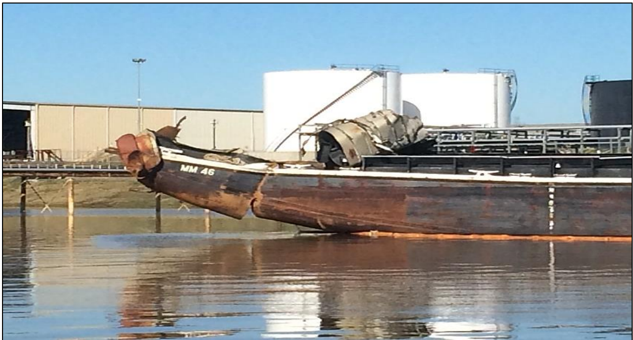
Damaged port bow of barge MM-46 . (Photo by US Coast Guard)
