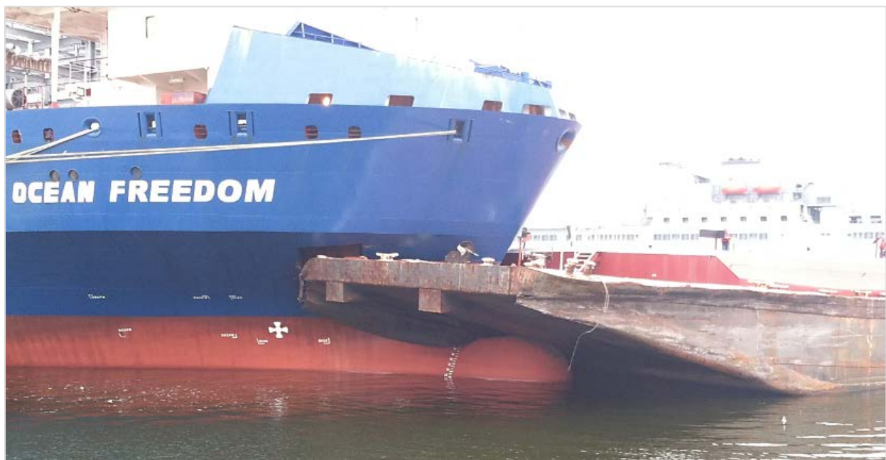
Impaled by the bow of the Ocean Freedom , the starboard bow of the Kirby 28044 is lodged just above the vessel's bulbous bow. In the background is the USNS Benavidez . (Photo by Coast Guard)
