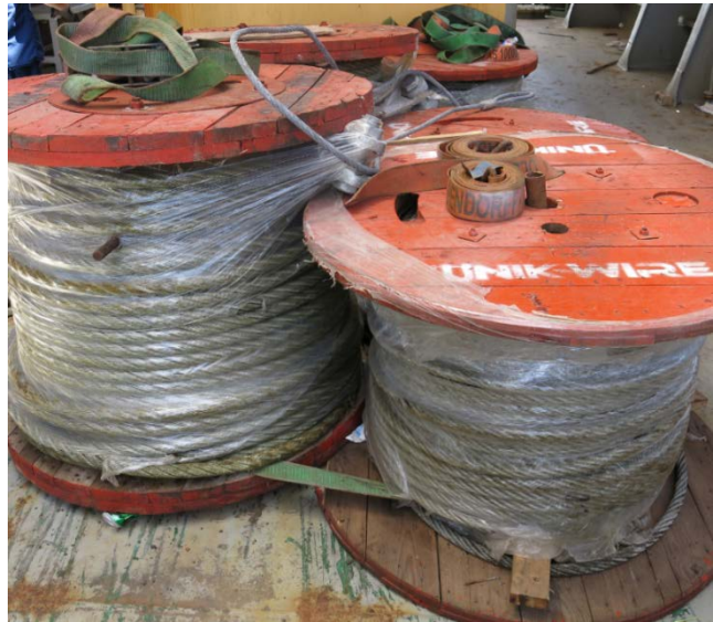
Coils of wire rope found on deck, photographed on July 9, 2015: at left, larger coil for the lifting wire; at right, smaller coil for the luffing wire.
