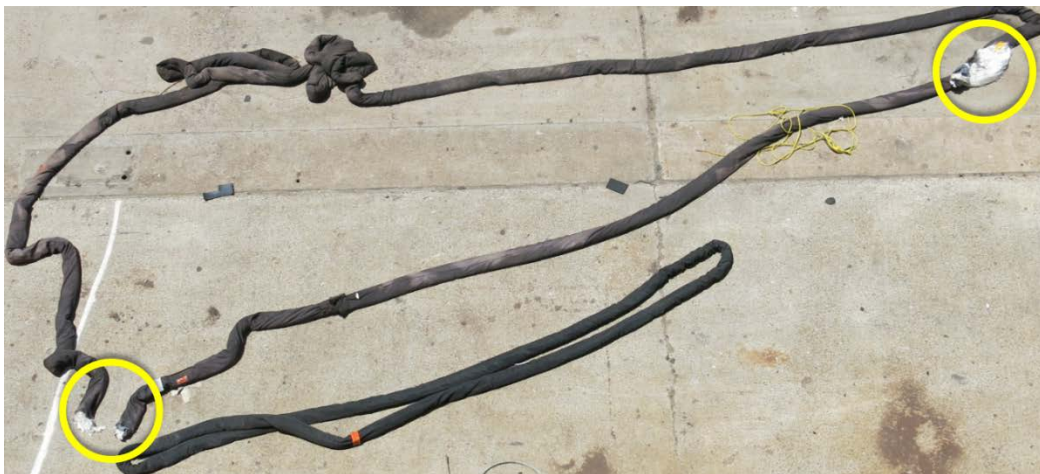
The long and short slings from crane no. 3. The area where the long sling separated is circled on the lower left; the section that sustained the abrasion and tears is in the upper right corner.
