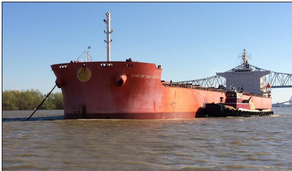
Star of Abu Dhabi after the accident, with missing port anchor. (Photo by US Coast Guard)
