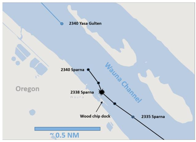
Track of the *Sparna* as the bulk carrier approached the wood chip dock and grounded. Times are rounded to the nearest minute. (Background by Google Maps)
