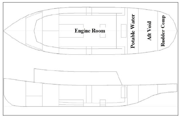
General arrangements, annotated by the Coast Guard Marine Safety Center, for *Spence* stability study. Shown are compartments extending aft of midship beneath the main deck. (Provided by US Coast Guard)
