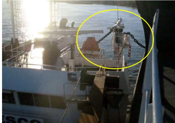
Left image shows Manizales cracked gear box. Right image shows Zen-Noh Grain Pegasus port anchor chain draped across Manizales crane and lifeboat. (Photos by Coast Guard and Zen-Noh Grain Pegasus crew)
