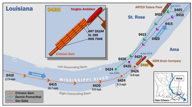
Based on automatic identification system data, the tracklines of the vessels *Crimson Gem*, *Dennis Fromenthal*, and *San Saba*, along with the position of the moored *Yangtze Ambition* in the river bend in Ama, Louisiana, leading up to the collision at 0430.
