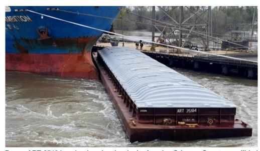
Barge ART 35184 wedged under the dock after the Crimson Gem tow collided with the bulk carrier Yangtze Ambition. (Photo by Coast Guard)
