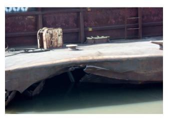
Damaged starboard bow of barge *XL* 359 from the *Crimson Gem* tow. (Photo by Coast Guard)
