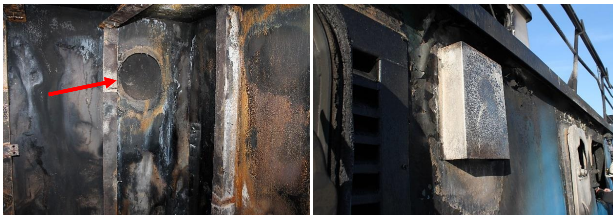
At left, the opening where exhaust fan had been mounted inside lavatory. At right, heat damage to painted surface of exterior bulkhead around exhaust ventilation duct.
